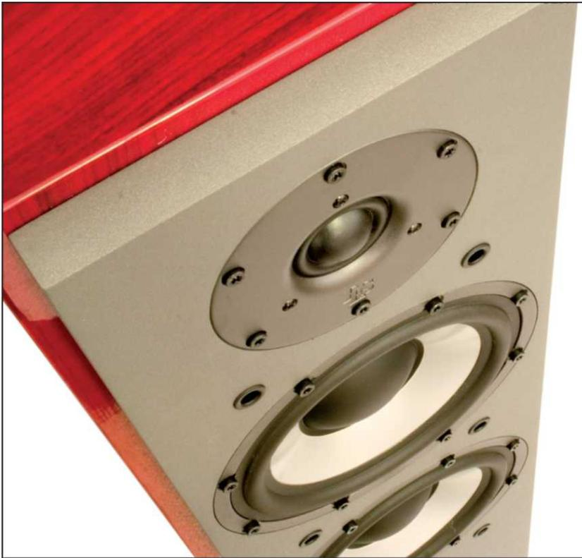
The speakers are attached with heavy duty fasteners, and the thick grey front panel appears to be of a vibration damping composition. The tweeter of the 2.5-way speaker is a 28 mm soft dome, the woofer/midrange and woofer speakers are both 6.5" aluminium diaphragm speakers. The single cable connector is a gold-plated, screw-clamp type.
